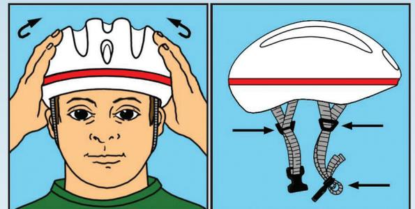
**Make sure the helmet fits snug and does not obstruct the field of vision. The chin strap should fit securely and the buckle must stay fastened.**
